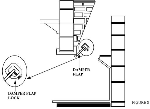
(5) Any chimney damper must be fixed in a manner which will maintain the minimum permanent vent opening at all times.
